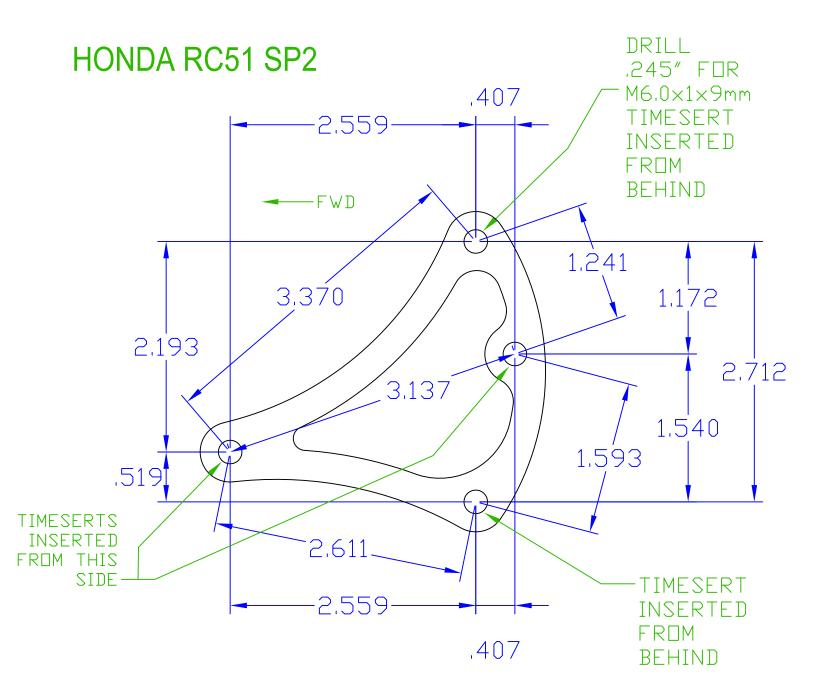
ADAPTER PLATE FOR FH012AA 1/4" CARBON FIBER PLATE
